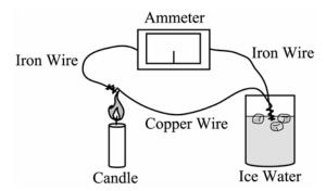
As the temperature difference between the ends of the wires increases, the current in the circuit
